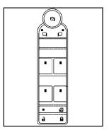
The power window switches are located on the driver's door.
